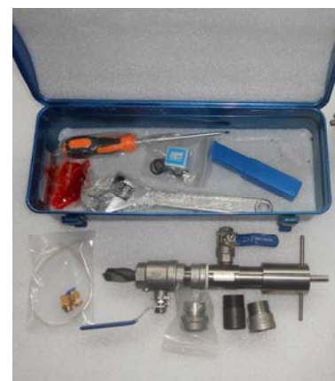
Hot taping driller
