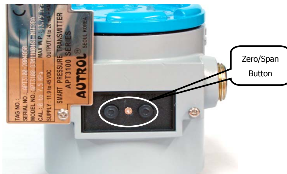
[Figure 3-4 Transmitter's Zero/Span configuration Button]
