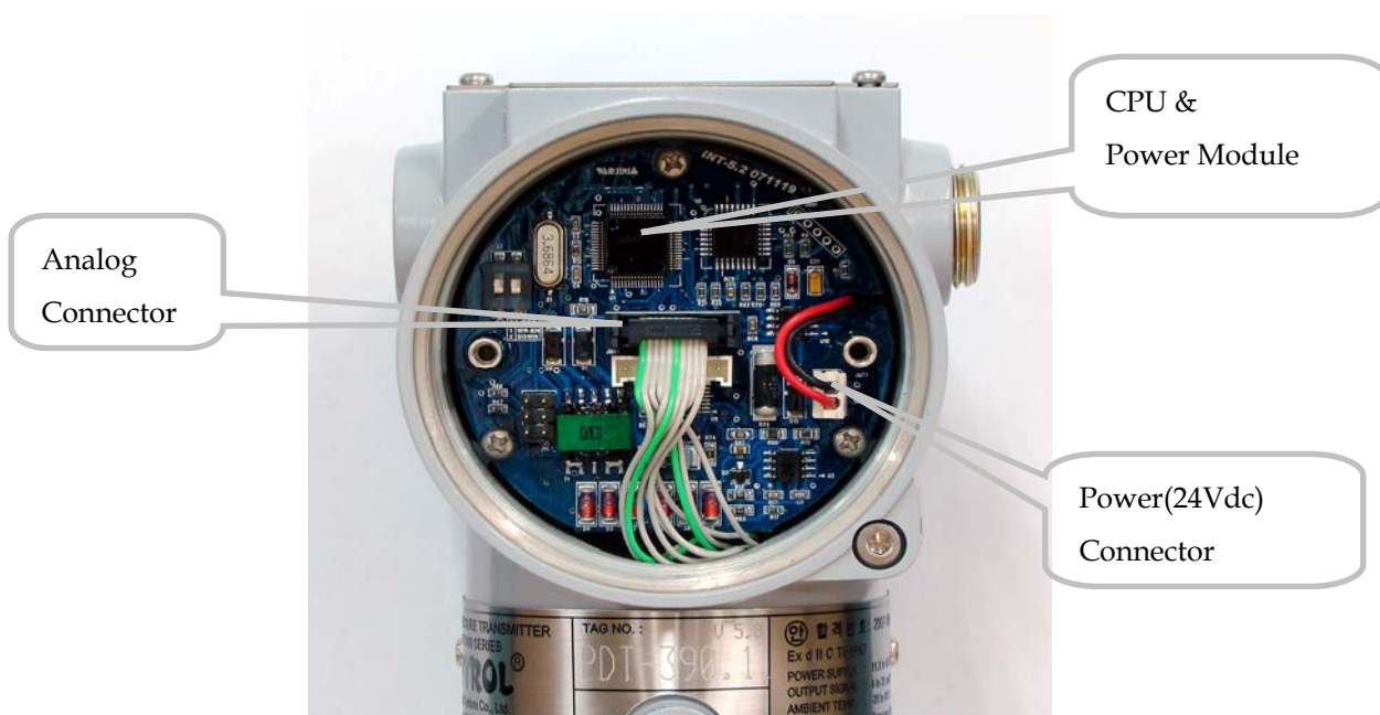
Figure 6.3 Structure of Electronics Module inner Transmitter
