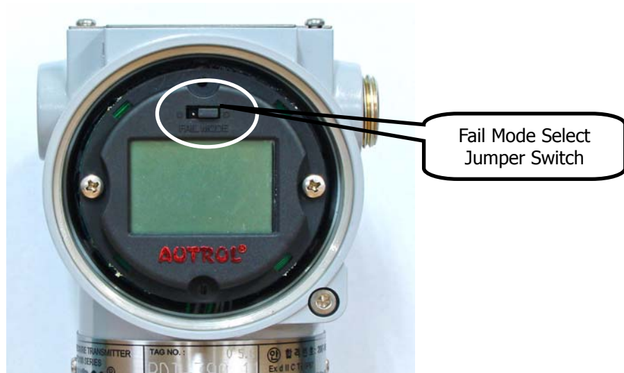
[Figure 3-2 LCD Module's Fail Mode Select Jumper]
