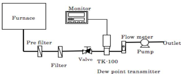
You can install TK-100 directly to a measurement bath like clean booth or a room, which needs to be humidity controlled.
