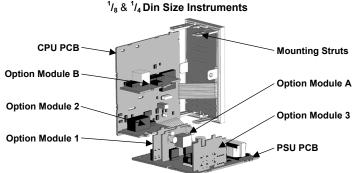
To access modules 1, A or B, first detach the PSU and CPU boards from the front by lifting first the upper, and then lower mounting struts. Gently separate the boards.
