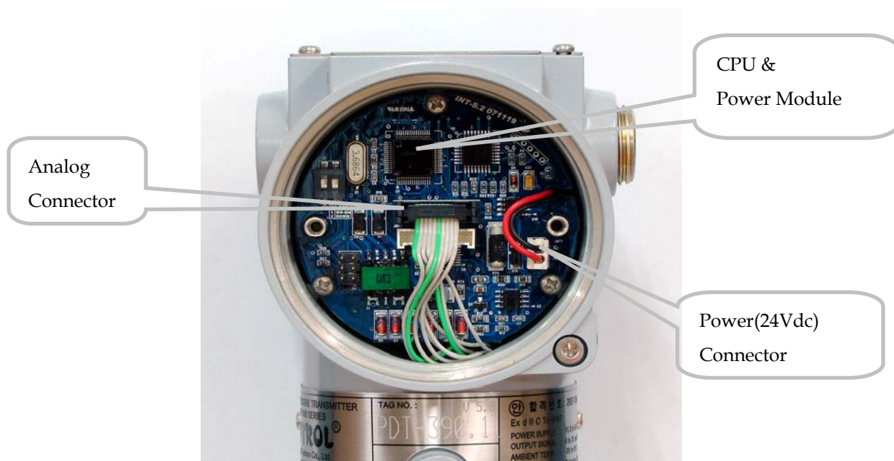
Figure 6.3 Structure of Electronics Module inner Transmitter
