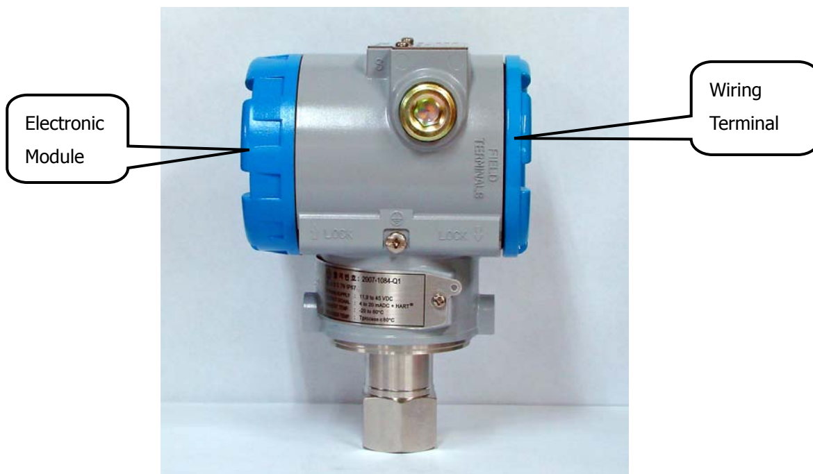
[Figure 6.2 Structure of Housing]
