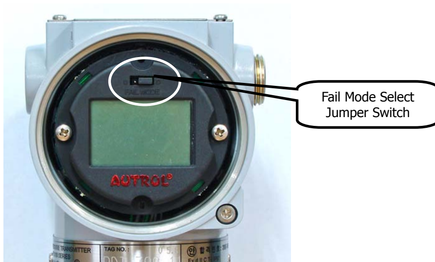
[Figure 3-2 LCD Module's Fail Mode Select Jumper]
